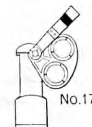
DWARF SIGNAL. Color. YELLOW light at night. Indication. PROCEED with CAUTION. Name. CAUTION Signal.
